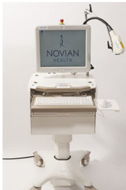
Novilase is an interstitial laser therapy system to treat breast tumors. The hope is that it will replace lumpectomy procedures as a minimally invasive standard of care for the removal of small tumors.
